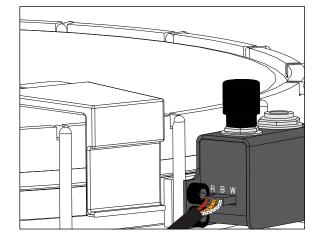
7) Wire it up Route the cables as shown by paying attention to the color codes marked on the pickup and battery holder PC Boards.
