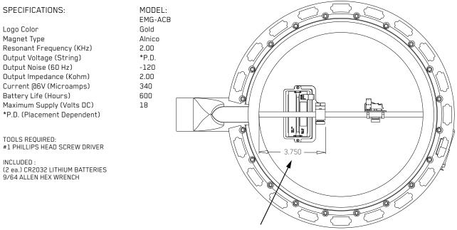
The "Sweet" Spot From both sound trials and experiments it's been determined that a distance of 3.750 inches (95mm) is about the best spot for the pickup.
