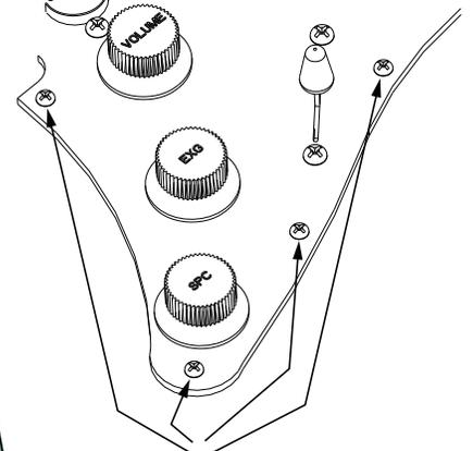
Battery Replacement: Remove these 4 screws, gently lift the pickguard' remove and replace the battery.
