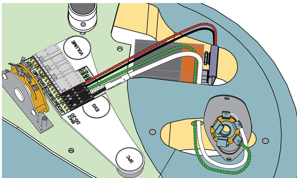
Route the Output Cable and Green wire from the Output Jack Cavity to the Control Cavity and plug them onto the BLK,WHT and GRN pins on the PC Board.
